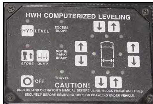
Figure 9-5. HWH Computerized Leveling System
