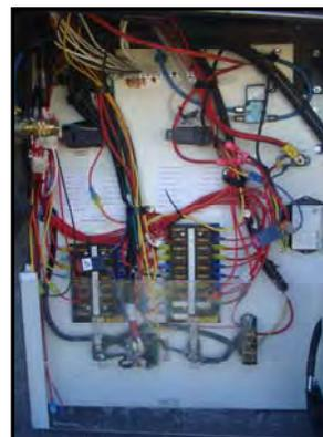
**Figure 7-15. Fuse Blocks in exterior compartment on driver's side**
