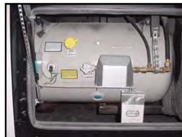
Figure 2-5. Liquid Propane Tank
