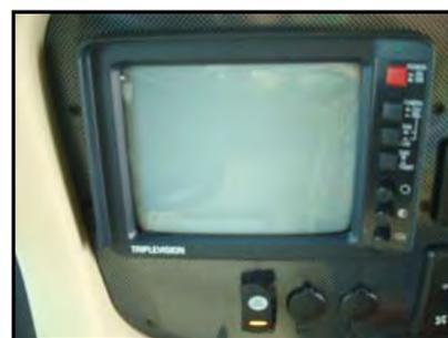
Figure 4-19. Rear-View Camera Monitor System
