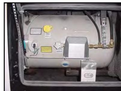
**Figure 3-4. Liquid Propane Tank**
